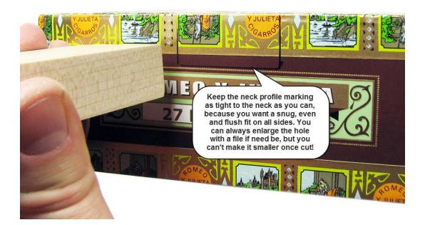
10. Once you have marked both sides of your box, it is time to cut the openings. It is recommended that you use a small saw, such as a coping saw, for this, but make do the
