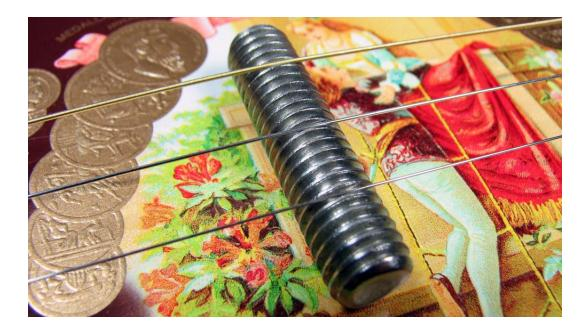
34. The threaded rods used for the nut and the bridge help you guide the strings into proper locations with the right spacing between them. The bridge should be placed about 2 ¾" from the bottom edge of the box. A 4-string instrument's strings will be proportionately closer together.
