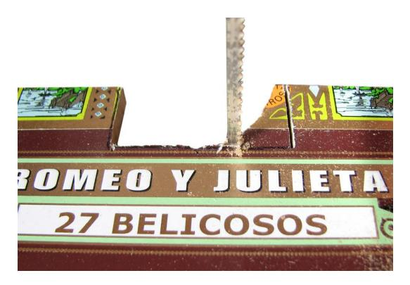
11. Once cut, test the fit of your neck , and if necessary use a wood file to carefully enlarge the cutouts. Ideally, you want the neck to fit very snugly and to be flush with the top of the cigar box
