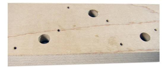
30. Once you've marked the screw locations, remove the tuners and pre-drill the holes with a 1/16" bit, then mount the tuners using the included screws. The finished tuners should appear as in the photo below. Note that your kit may have included two tuners for the right side of the headstock (when looking from the back), instead of the two on the left as shown in the photo, or if it's a 4-string kit there will be 4 total tuners.
