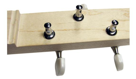
31. Now it is time to file a groove for the nut to rest in. Mark a pair of parallel lines about ¼" from the edge of the headstock tuner cutout, and then use a round file to file a rounded groove into the neck, as shown in the photos below. This groove will help keep the nut in place once the guitar is strung up. You can lower the action of the instrument by deepening this groove as desired.
