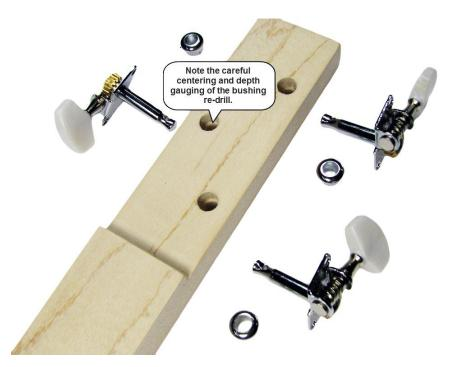
29. Now it is time to insert the tuners (gear towards the body!) and mark the holes. You absolutely must pre-drill the screw holes using a 1/16" bit. If you just try to force the delicate screws into the hardwood without pre-drilling, they are almost guaranteed to sheer off. Make sure that the tuner edges are parallel to the headstock edges, and then mark the center of each hole location with a sharp pencil or fine-point marker.
