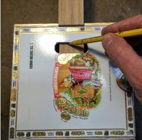
After you remove that space in the lid, trace the top edge onto the neck underneath.
