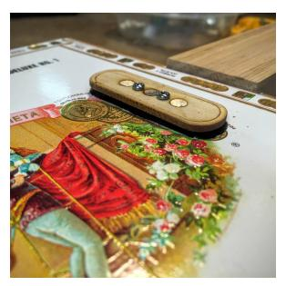
Install the mounting screws, securing the pickup to the neck.
