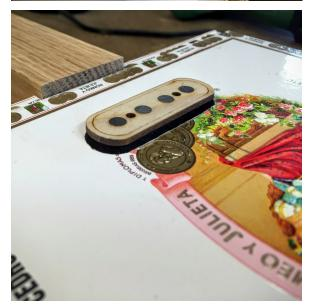
Once the wood blocks have been installed, set your pickup in the recess, making certain to line it up with the space cut out of the box lid.
