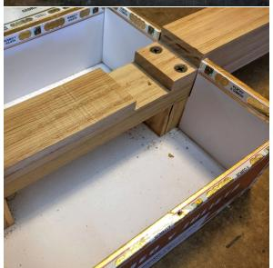
Remove the space at your determined depth between the lines you've drawn on top of the neck.
