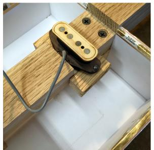
You can also use the 2 outside holes in the bottom plate of the pickup to mount it onto the neck.
