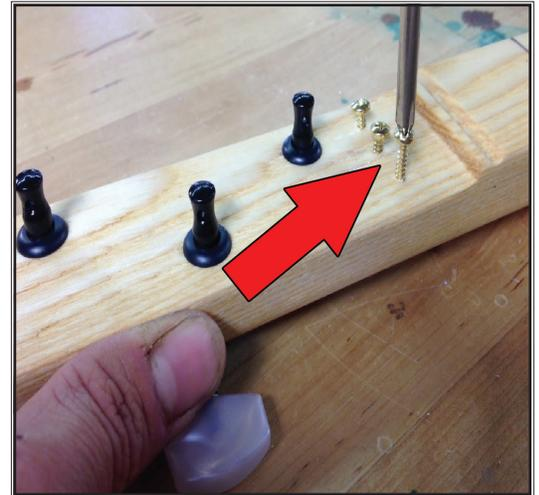
*Suggested placement of the string retainer screws on the headstock.*
