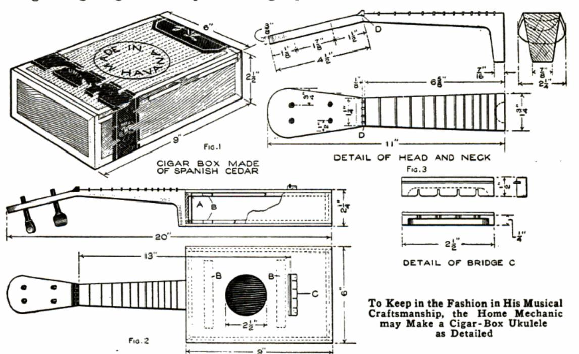
animal glue, should be done after the bridge C is in place, and the other parts are made. The bridge is of hard wood hollowed underneath the notched edge, as detailed, and is fitted with a metal string contact.
