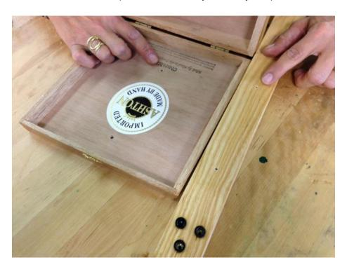
Open up your box and with the box hinges facing the headstock and your newly installed tuners, line up the holes in the box lid to the holes on the neck. Wielding your trusty Phillips head screwdriver twist those two ¾" lath screws (**Part "F"**) into place. Your box is now firmly secured against your neck.
