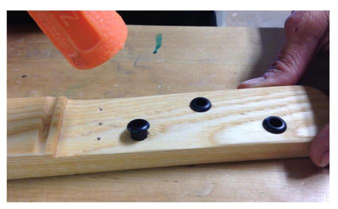
While you have the neck facing up, insert your three brass screws (**Part 'E'**), one at a time, into the three holes that are in a line with one another at the base of the headstock. They are located under the bushings you just installed and just above the groove that has been filed out for the nut, and are visible to the left of the bushings in the photo above.
